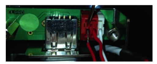
Once the connection is made it can take approximately **45 seconds** to **one minute** for the PDF Logger to display the temperature on the LCD. The temperature probe connection is non-polarized as the red wires can be switched.
