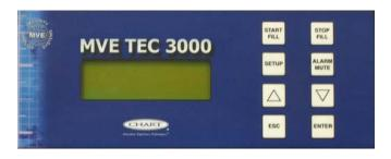
The TEC 3000 employs a variety of high level features that enable the controller to monitor and control the environment inside a freezer with a high level of precision.
