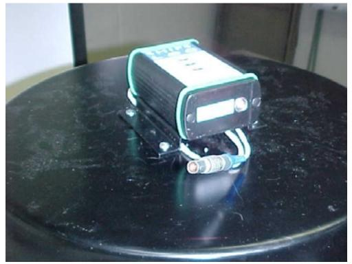
One of the many features of this data logger is it can be disconnected from the temperature probe when temperature monitoring is not required.
