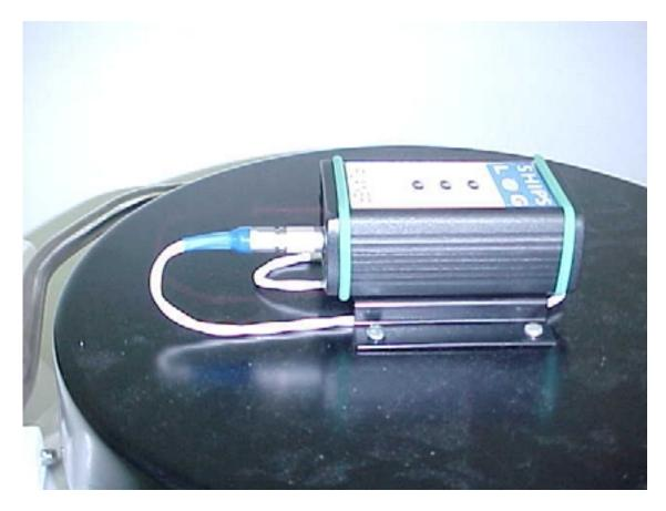
The logger is programmable by the user via PC software and can be initiated via a magnetic key, which can be shipped separately from the vapor shipper.
