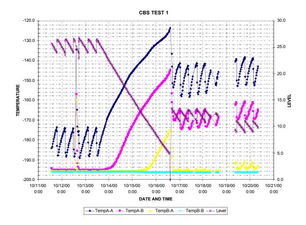
This graph shows the fill cycles and level and volume relationship within a test submerged chamber system in MVE's development department. Note the fill cycle times and the relationship of the top box temperature and level, and the subsequent failure of the isotherm as the level falls lower. Note also that the total time period for the top box to reach and exceed the critical temperature is less than 4 days.
