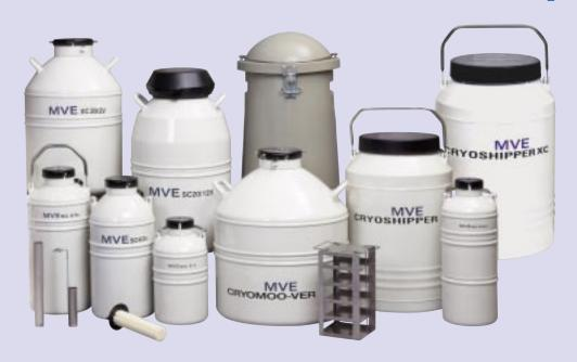
MVE Vapor Shipper containers are designed for the safe transportation of biological samples at cryogenic (-150°C or colder) temperatures. Fabricated from durable, lightweight aluminum, they employ a hydro-phobic absorbent that contains the liquid nitrogen for "spill free" shipping. The absorbent also repels moisture and humidity, assuring the maximum holding time. This eliminates the necessity to dry units between uses.
